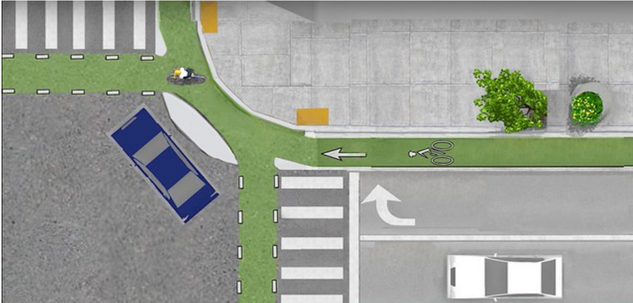
FIGURE 3. EXAMPLE OF A PROTECTED INTERSECTION TREATMENT TO MITIGATE CONFLICTS BETWEEN RIGHT TURNING VEHICLES AND PEOPLE BIKING
